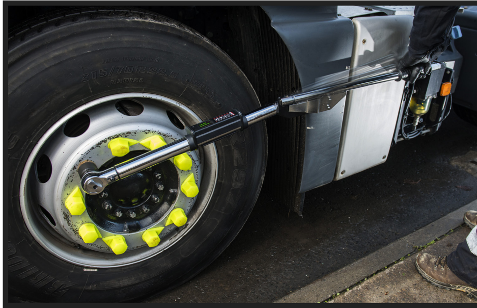
An SB750S breaking over at set torque
